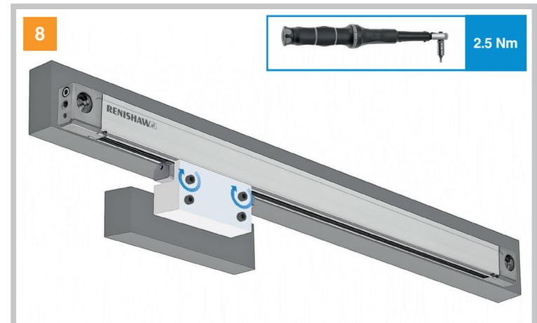
Using the correct tool, tighten the screws to a torque of 2.5 Nm.
