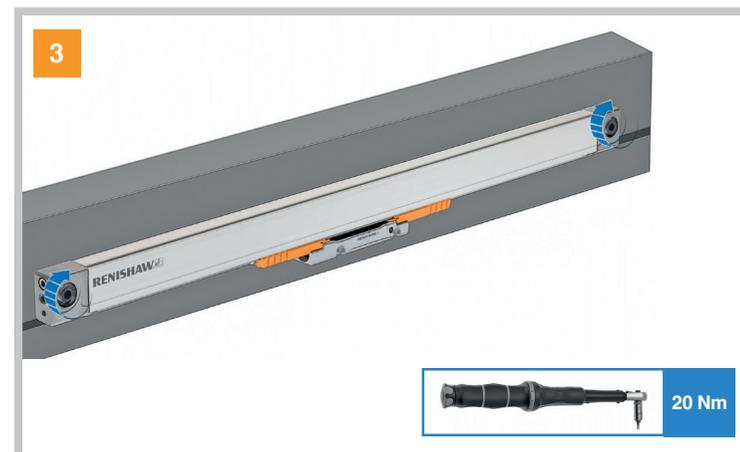
Tighten to a torque of 20 Nm.
