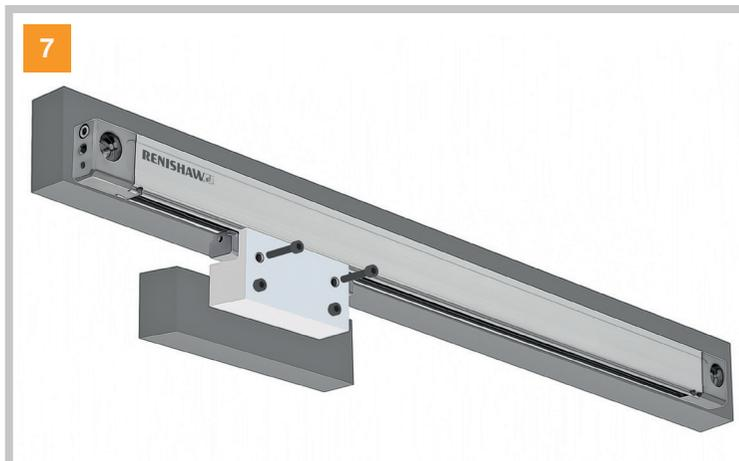
Align the readhead with the readhead mounting bracket and secure with M4 screws and nuts.
