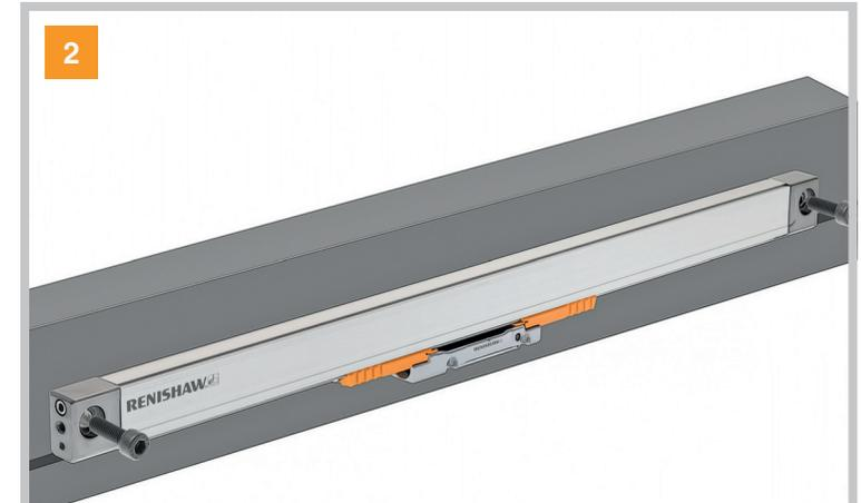
Loosely secure the extrusion to the mounting surface with the two supplied serrated washers and M8 screws placed in the end cap mounting holes.
