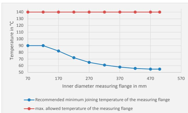
\*The temperature specification refers to an ambient temperature of 22 °C. If the ambient temperature is different, adjust the assembling temperature accordingly
